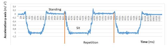
Figure 5. Acceleration in the *Y*-axis direction during the legs strength test.
